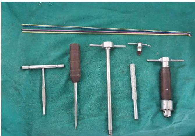
Figure [1]: The equipment needed for inserting elastic nails and the accessibility of titanium nails in different sizes
